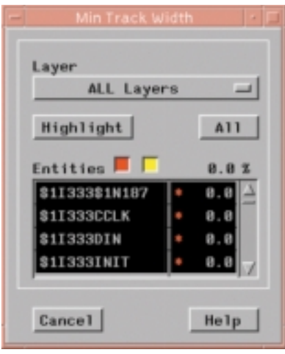
Figure 7. A dialog box showing the various entities in the design that violated the "Min Track Width" guideline.
