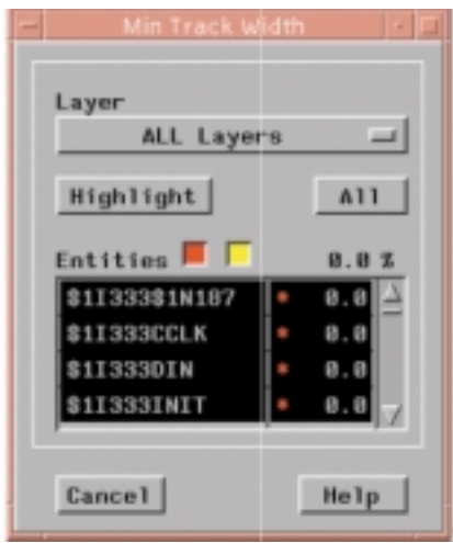
Figure 6. The Visula Design Adviser interface showing the results of an analysis of a PCB design using the guidelines implemented earlier.
