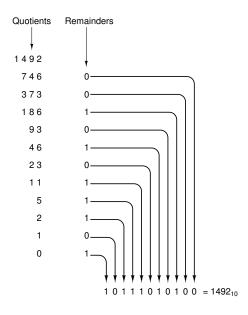
**Figure A.5** Conversion of the decimal number 1492 to binary by successive halving.
