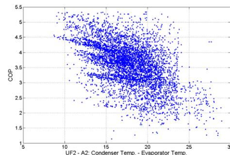
Figure 1: Original Data for Heat Pump COP vs A2
