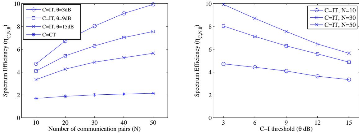
Fig. 5. Comparison of the spectrum efficiency ( $\eta_{C,N,\theta}$  = number of communication pairs where acceptable communication can be sustained (C-I threshold =  $\theta$  dB) per channel) using Cautious binary transmitter-centric constraints (CT) and Interference Temperature based non-binary receiver-centric constraints (IT) for channel assignment in a CR network with  $N$  communication pairs.
