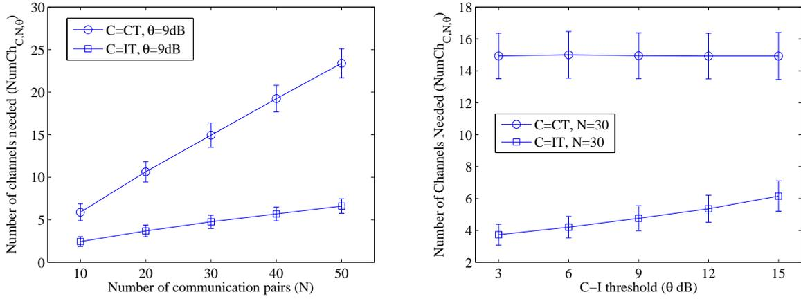
Fig. 4. Comparison of the number of channels needed ( $NumCh_{C,N,\theta}$ ) to ensure acceptable communication (C-I threshold  $\theta$  dB) amongst  $N$  communication pairs using Cautious binary transmitter-centric constraints (CT) and Interference Temperature based non-binary receiver-centric constraints (IT) for channel assignment in a CR network.
