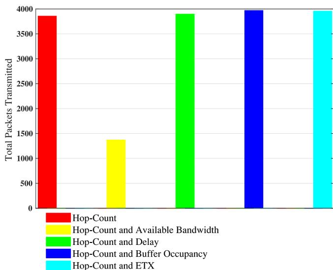
Fig. 5. Total packets transmitted using null RDC.
