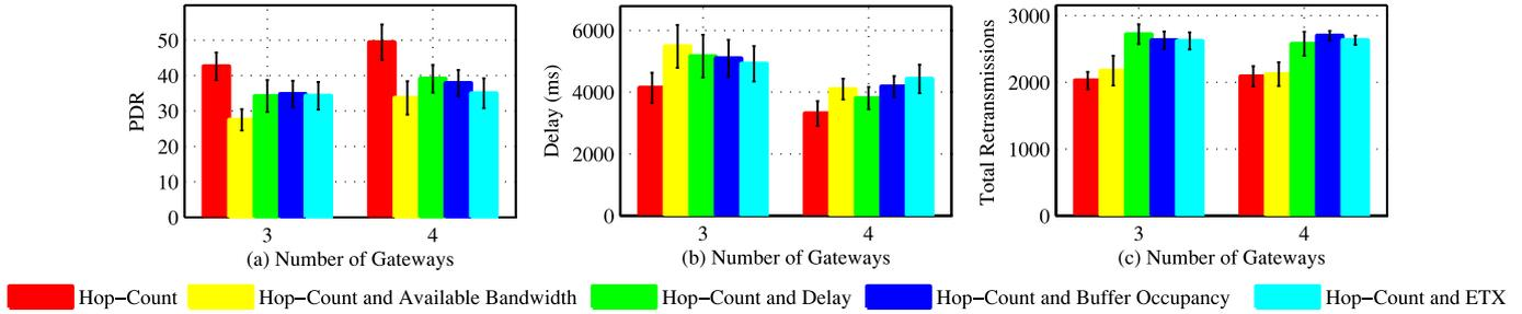
Fig. 13. RPL-based protocol performance using a greedy approach and increased data generation (ContikiMAC).
