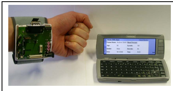
Figure 4. A Tyndall-DMS-Mote attached to a patient's wrist. Pulse rate readings are sampled and returned to the DMS-Server for real-time Validation. Here the Nokia 9500 is utilised to transfer data back to the DMS-Server.
