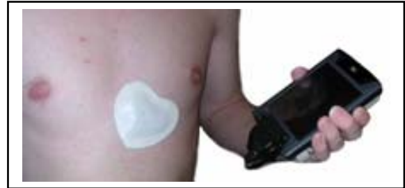
Figure 5. The WPR wireless ECG-sensor attached to a patient's chest. It is transmitting vital sign recordings to the DMS-Server through a Hand-Held-Device.
