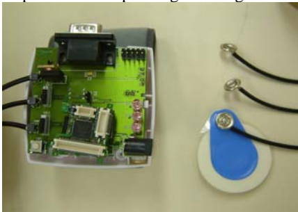
Figure 2. Wireless Patient Module with miniaturised Tyndall mote
