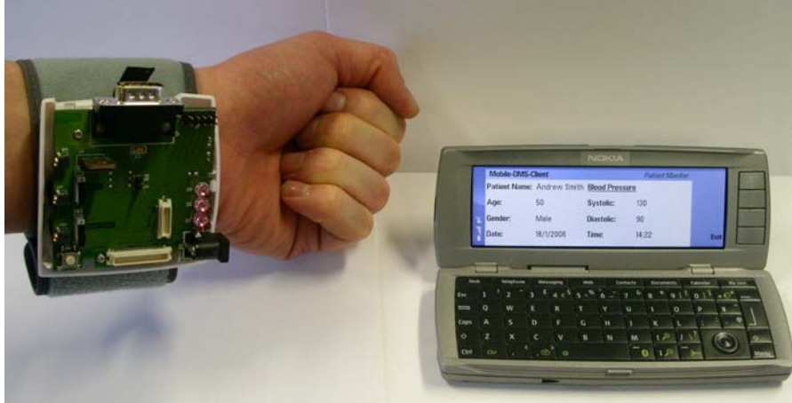
Figure 2. An Exposed Tyndall-DMS-Mote prototype and Mobile-DMS-Client (i.e. Jade-Leap agent on a Nokia 9500) displaying blood pressure readings and patient details.
