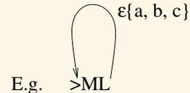
$TM$  is executed. When it would halt, if the test is true, it returns to state  $q_0$  instead. In the example, the machine moves left repeatedly, for as long as there is an  $a$ ,  $b$  or  $c$  under the read/write head. When the symbol under the read/write head is not one of  $a$ ,  $b$  or  $c$ , it halts. It is usual to include a test, otherwise you have an infinite loop.
