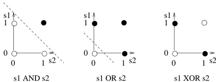
We have two inputs, which can be 0 or 1, drawn on the axes. Black dots indicate points in the input space where the output should be 1. But a TLU outputs 1 iff some threshold is exceeded, so this space is divided into two (those points where the weighted sum is above the threshold and those points where it isn't). So, in the cases where we can draw a straight line that separates the white dots from the black dots, we can use a TLU.
