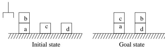
The robot is capable of four actions: stacking a block that it is holding on top of another block; unstacking a block from another block; picking a block up from the table; and putting down a block that it is holding onto the table.
