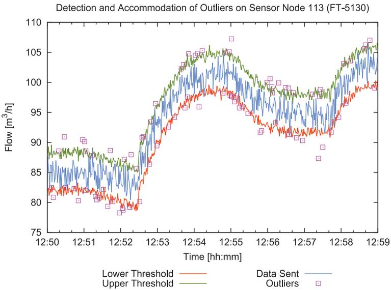
Fig. 26. Outliers detection and accommodation at node level.
