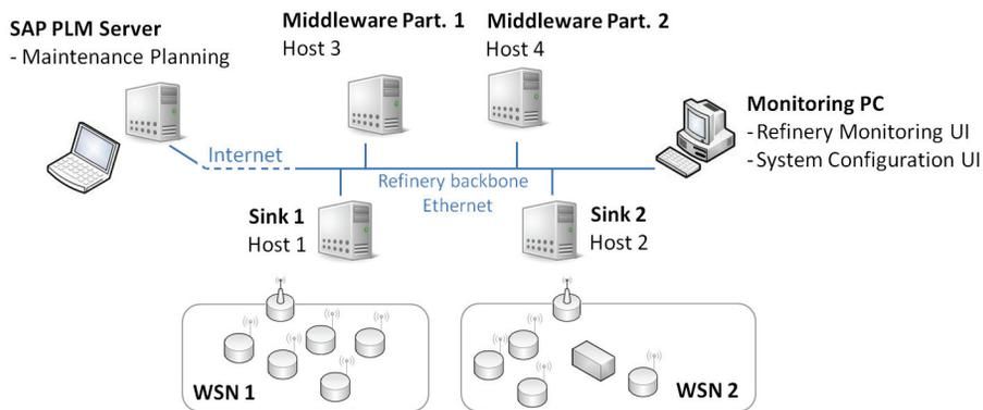
Fig. 7. The GINSENG deployment setup also includes middleware, backend, and frontend applications.
