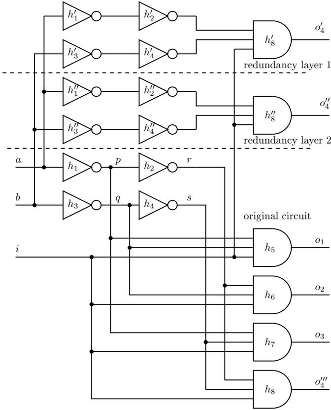
Fig. 4. A triple-redundant demultiplexer circuit
