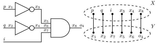
Fig. 9. A circuit and its interconnection bigraph
