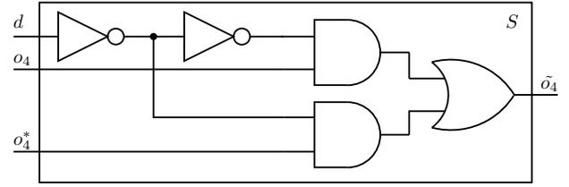
Fig. 7. Example of an output selection circuit
