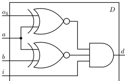
Fig. 6. Example of a danger detection circuit
