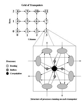
Figure 1. Network of transputers and the structure of individual processes
