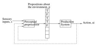
The inputs to the perceptual preprocessor are the agent's sensory inputs, s, the previous vector of truth-values, p, and the action the agent has just executed. In pseudocode, the agent does the following at each point in time:
