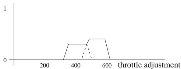
We must now determine a precise throttle adjustment value. This is the process of *defuzzification*. There are many approaches but a common one is the *centroid method*. The centroid will be the throttle adjustment value at which a vertical line would pass through the centre of the set (equal areas to left and right of the line):
