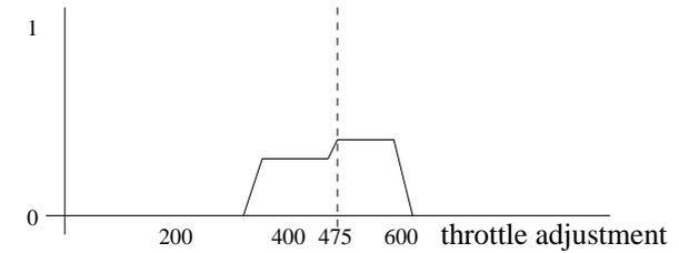
Finally, the agent is ready to *act*. It sends a signal to its throttle requesting an adjustment of 475 (as computed by the centroid method). And now the cycle begins again.
