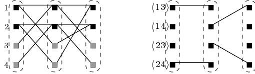
Fig. 4. The first graph shows the microstructure of a simple CSP, three variables and four values each, allowed combinations are linked. P is super AC since the super domains are of size 2 (black values), and the repair domains are of size 4 (black and grey values). The second graph shows P \times P , which is not arc-consistent.
