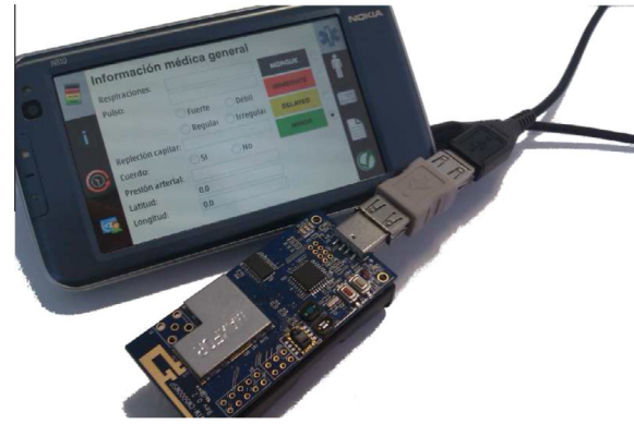
Fig. 5. A WSN node connected to a Nokia N810 handheld.
